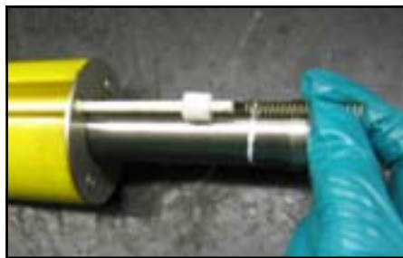
5. Remove control rod bottom stop, spring and top stop
