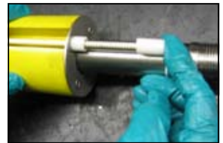
6. Refit top stop, fit new spring and refit the bottom stop.
