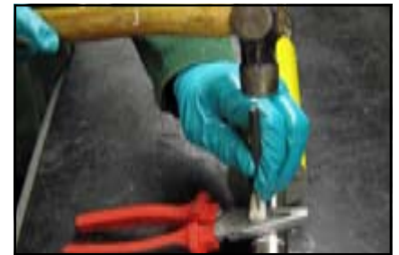
3. Push pin out with 1.5mm punch
