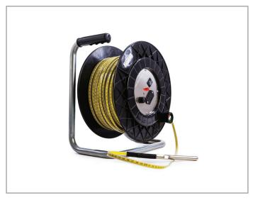
Water Level (Dip) Meters are used to determine the water level within a borehole, piezometer pipe or sump. They consist of a stainless steel probe which is specially designed to minimise displacement errors providing unparalleled accuracy, particularly within small bore piezometer installations. As the probe is lowered into the water a single audible buzz is heard and an LED light shows.
