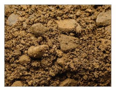
20mm "as dug" ballast/sand & gravel mixed aggregate can be used as an 'all-in-one' aggregate with cement and water to produce coarse concretes.
