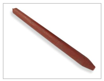
Loop Weights are used to aid the installation of Thermo-Loops® in deep boreholes, difficult ground conditions, tight boreholes or where the viscosity of the borehole fluid means that the loop will not fall under its own weight.
