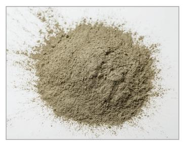
Grout Mix is a pre-blended powder mixture of premium grade high quality sodium carbonate activated Bentonite powder and Ordinary Portland Cement (CEM 1) in a ratio of 2:1.
