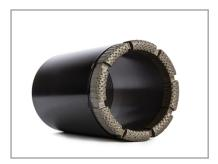
Used for drilling soft, abrasive, unconsolidated formations that are not effectively drilled by impregnated diamond bits. They can also be used for drilling harder formations with low powered drills, where the rotational speed or bit load produced is not sufficient to run impregnated bits.
