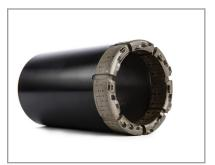
Recommended for coring soft to medium hard, abrasive and fragmented formations, giving a high percentage core recovery even where there are rapid changes in formation hardness. The cutters are stable at high temperature and are therefore suitable for air flush drilling, as well as water, mud and foam.
