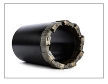
Recommended for coring soft to medium hard formations, with water, air, mud or foam as the flushing medium. Ideal for air flush applications where a high rate of production is required.
