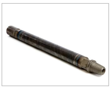
Friction-welded rods have friction welded tool joints which are specially hardened and made of the highest quality steel. This means that different steel qualities can be chosen for the mid-body section and the tool joints. A high-quality alloy steel is used for the tool joints, increasing the strength of the threads where it is required, combined with a thinner tubular material in between. This makes the rods lighter and easier to handle.
