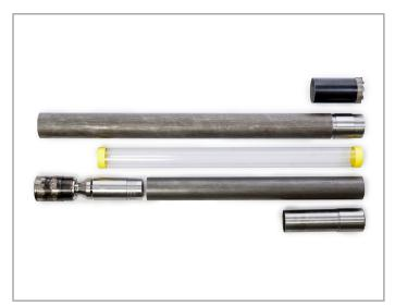
The T2 series is a range of components which produce 42, 52, 62, 72 and 84mm cores suitable for medium to hard geology. These core barrels have a relatively small cutting area and therefore permit rapid penetration, especially in harder rock formations. The thin wall barrels and core bits produce fewer cuttings which permits the use of lower flush velocities resulting in diminished sample disturbance. Water or polymer flush is required.
