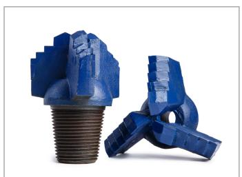
Three-winged step drag bits are available either as a one-piece forged alloy steel construction or cast with Tungsten Carbide cutting tips and gauge sides to ensure longer life. They are designed for air flush with central flushing ports.
