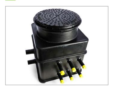
Type DC3 moulded manifold chambers are used in combination with geothermal manifolds. They provide security as well as a central location for controlling and monitoring the flow and pressure of geothermal ground source heat recovery systems. Moulded from tough, 11mm thick, solid walled polyethylene, they are available in various sizes and inlets and outlets options together with accessories such as control valves, flow meters, fill and bleed ports and pressure gauges.
