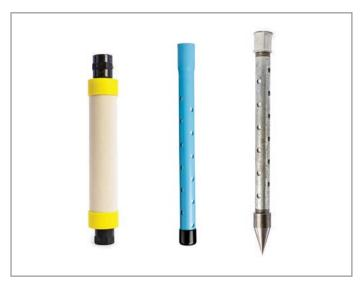
Casagrande standpipe piezometers are a simple and economic method for measuring groundwater pressures in soil and rock. They are made up of low air entry porous plastic or ceramic elements which are connected to standpipe tubing and lowered into a pre-drilled borehole. Alternative types may be driven or pushed into soft soil.
