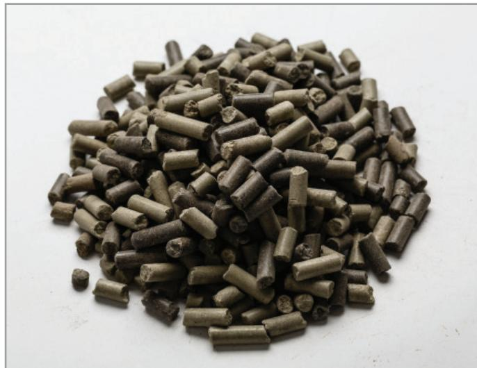
Bentonite Cement Pellets are used in construction, drilling and tunnelling projects for sealing applications where more strength is required than can be achieved with pure Bentonite alone. This product is used to seal off contaminated land, seal around pipes or tunnels, seal up bore holes, fill voids, protect pipes and cables in conduits or provide a more conductive medium for cable grouting.
